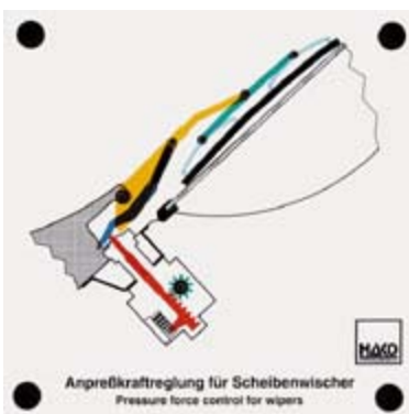
Order no. 397 Vertical force control of windscreen wipers
