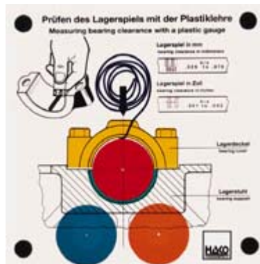
Order no. 249 Measuring bearing clearance
